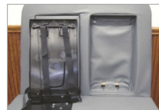
4 Lift out insert and belts as a complete unit.
