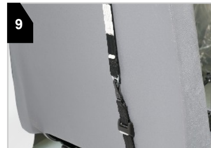
9 Hook top belt from step 3 to snap clip on bottom belt from step 6 together as shown. Adjust to create a snug fit.
