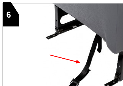
6 Pull belt and PCR to back of school bus seat. Belt should look as shown when finished.
