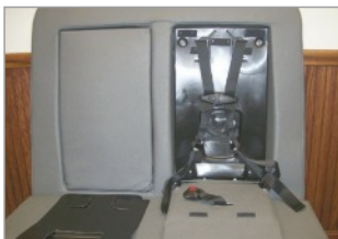
1 Open the front insert flap and remove seat pad.
