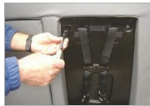
3 Locate and remove 2 nuts on each top corner of insert.
