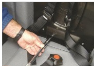
2 Locate and remove 2 nuts located in the middle of panel bottom.
