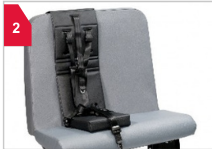
2 Unfold PCR and place on seat as shown.
