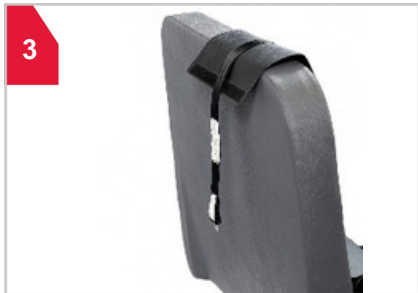
3 Drape PCR top belt over school bus seat back and let belt hang down.
